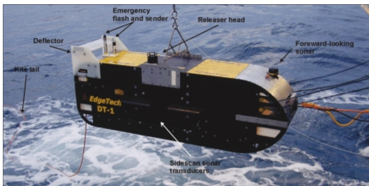
Figure 1: The DTS-1 side-scan sonar towfish during deployment.
