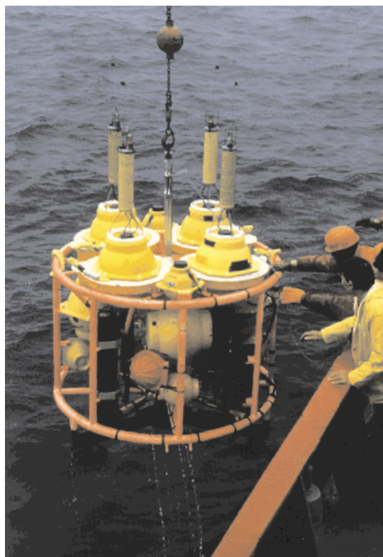
Vassie et al., page 14, Figure 2. MYRTLE (Multi Year Return Tide Level Equipment). This instrument is capable of 5 years continuous operation at depths to 6000 m. The measured pressure variations near the sea bed are returned by releasable data capsules annually.
