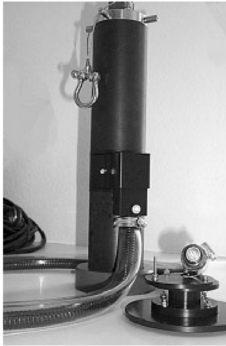
Fig. 1. Photo of the Benthofluor housed in a water resistant cylindrical case. The fluorometer is connected with a 5 m long optical fibre to the measuring head. The special disc-shaped measuring chamber is shown in the front. This chamber is placed on top of the sediment and connected to the fibre bundle prior to measurements.
