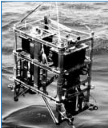
Figure 1. The Underwater Video Profiler (UVP) instrument package presented here includes the underwater imaging system, an SBE CTD, a fluorometer and nephelometer both from Chelsea Instruments.
