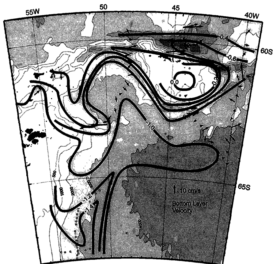
Figure 5. Bottom Water potential temperature of the lower 10 dbar of the CTD cast, if within 30 dbar of the seafloor (a station where the last scan is 30 dbar from the bottom would have a value that is the average of data 40–30 m from the bottom). Average velocity within the lower 120 dbar derived from (bottom referenced) LADCP data is shown as vectors. The majority of DOVETAIL stations approached within 10 m of the bottom. Temperature data from the 1992 Ice Station Weddell data set are included [Gordon, 1998] as shown by the open circles with no velocity vectors.
