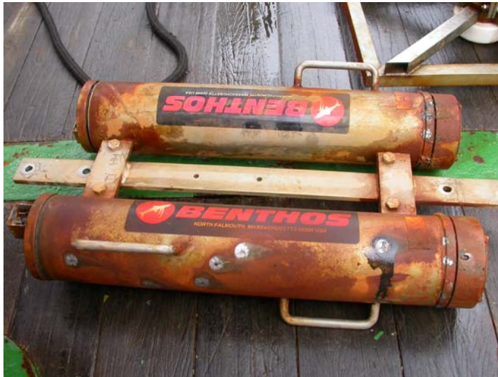
Figure 14: The heavily corroded video camera with discrete holes in the pressure cylinder.
