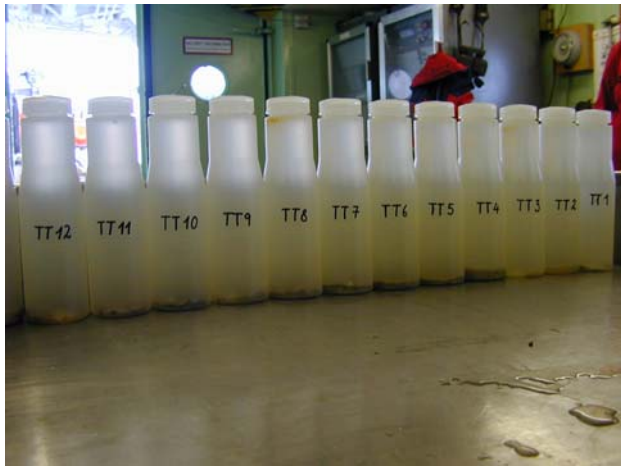
Figure 13: 13 filled sample cups (8 days sampling intervals) indicating seasonal changes in particle deposition.
