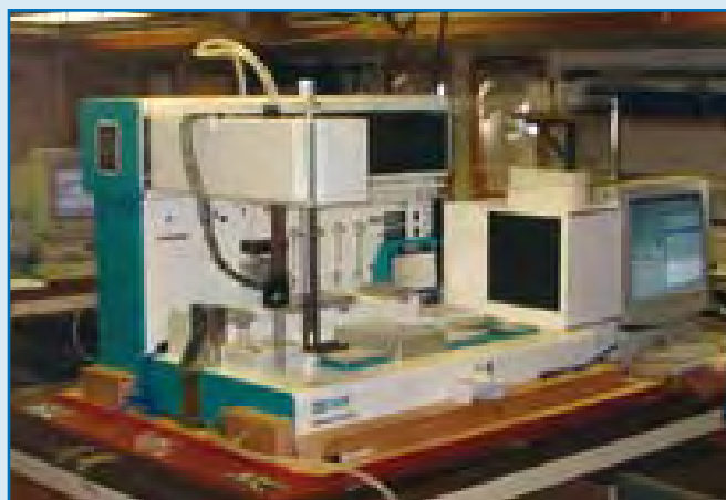
Figure 1. Robotic workstation onboard RRS Discovery. Conventional microscopy has been merged with molecular analysis to analyse Calanus species composition in the North Atlantic during the large-scale surveys of the Marine Productivity programme.
