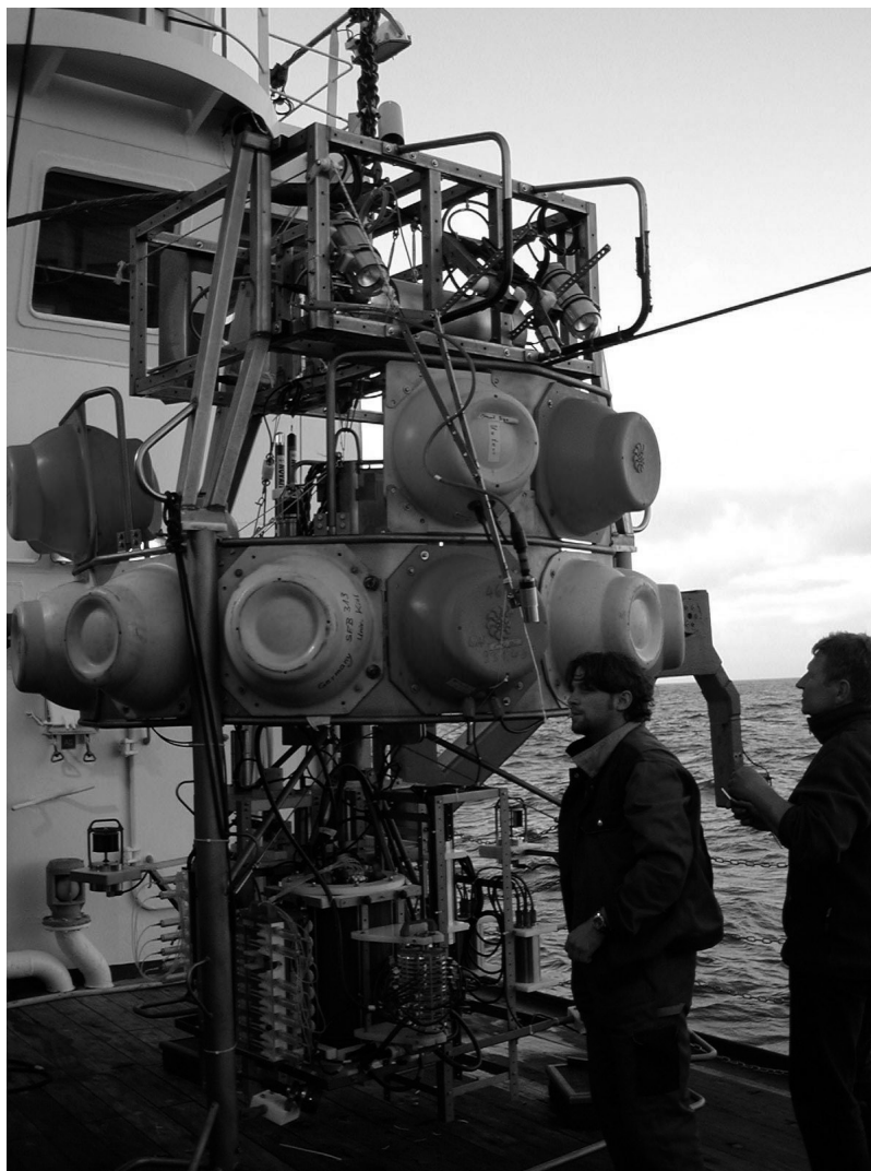
Figure 3. Biogeochemical observatory (BIGO) with launcher on top ready for video-guided deployment.
