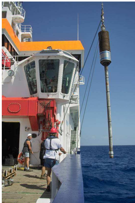
Fig. 5.4: GCPP deployment, the bottom of the corer weight houses the electronics package; rings visible around the corer provide guidance for the pipe connecting the pressure sensor to the tip of the corer;
