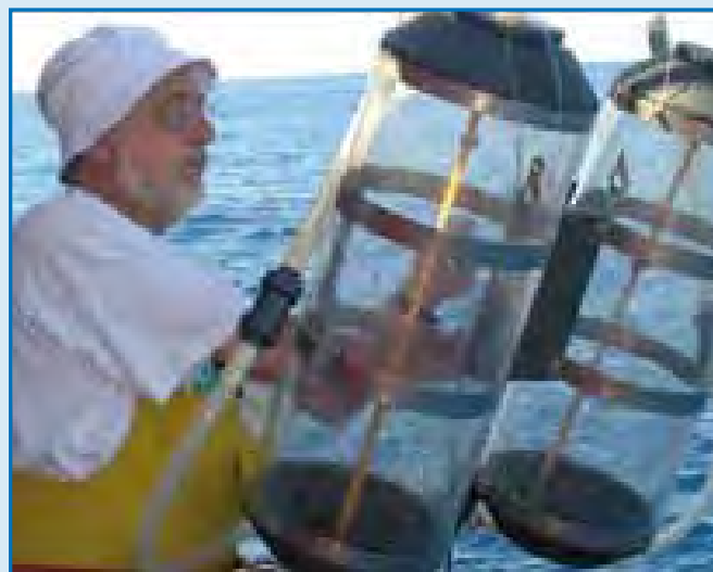
Figure 1. Large volume water bottles to take samples for zooplankton biomass.
