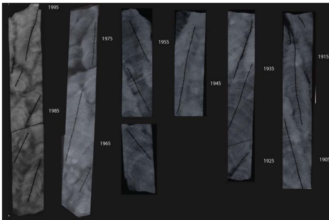
Figure 2.1b The X-Radiographs of core TH2. The dark lines are the sampling transects for stable isotope and trace element analysis.
