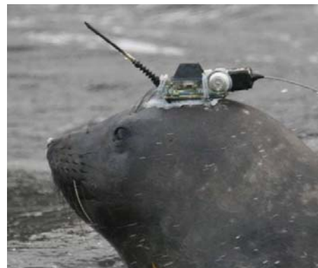
Figure 1: (a) An elephant seal equipped with a CTD logger. (b) Position of the profiles transmitted by the 16 CTD loggers deployed at Kerguelen in 2007.
