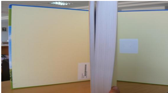
Figure 19. RFID tag and barcode used on a document
