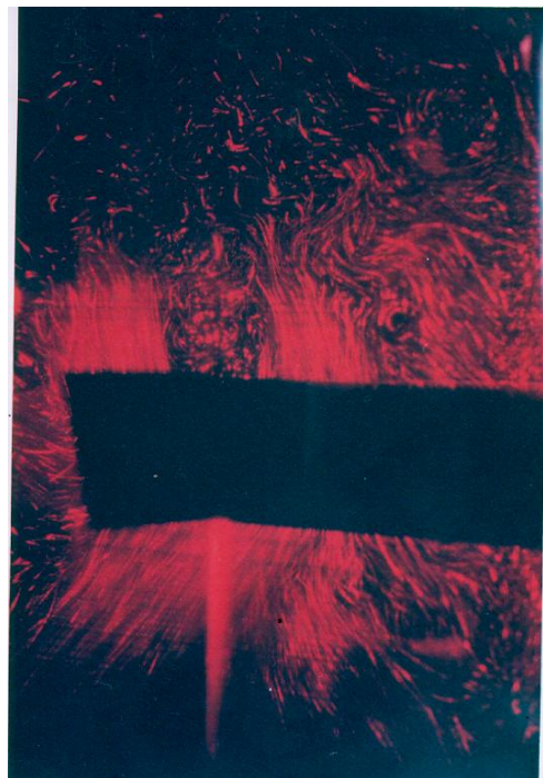
Fig. 4. Flow past V-gutter, limbs in line with inlets, X=50\text{mm} , V=60\text{ mm/s} , hydrogen bubble streak technique
