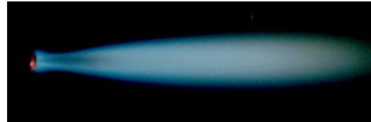
Fig. 8. Disc stabilised subsonic hydrogen diffusion flame
