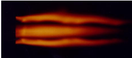
Fig. 6. Supersonic hydrogen diffusion flames (4 port injection)
