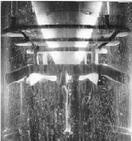
Fig. 10. Flow pattern - Flame stabiliser/ fuel ring assembly in optimum position
