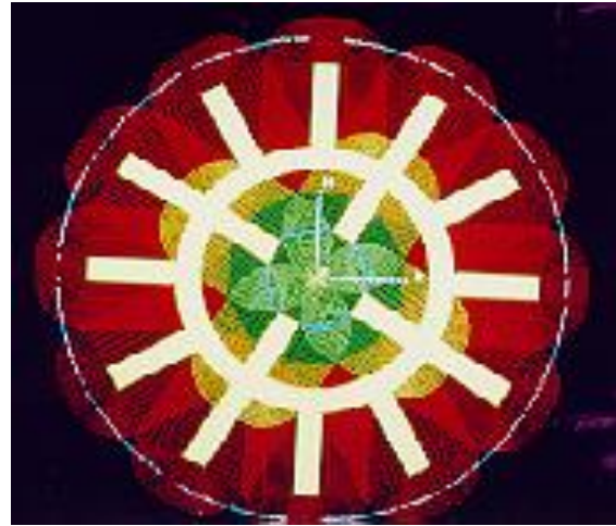
Fig. 7. Restricted flame growth - Ring with 12 outer radials and 4 inner radials, L/D = 1.4
