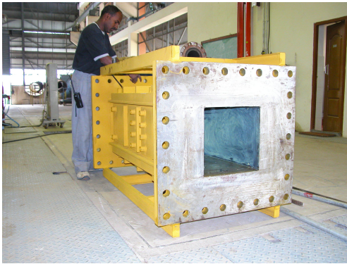
Fig.7 Mach 3.6 water cooled nozzle
