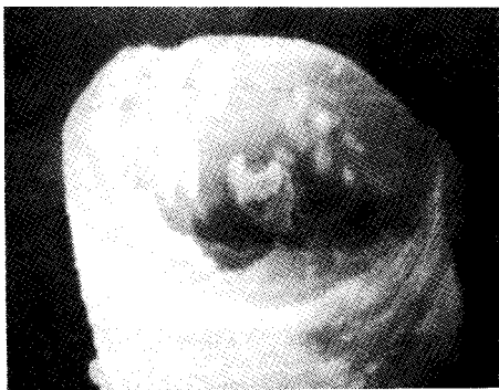
Fig. 5. Partial hollowness in a heat treated fibre.
