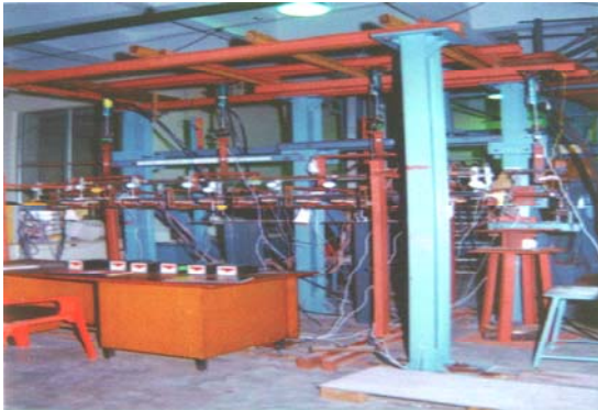
Fig. 31: SARAS LH Elevator Undergoing Static Testing 198% of Limit Load
