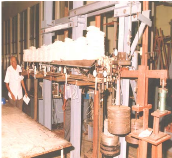
Fig. 29: Elevator LH Undergoing to 100% of Limit Load Test
