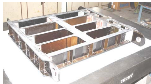
Fig. 3: A View of the Partial Assembly of the Wing Test Box
