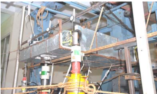
Fig. 13: Wing Test Box Enclosed in the Bag and the Insulating Outer Box
