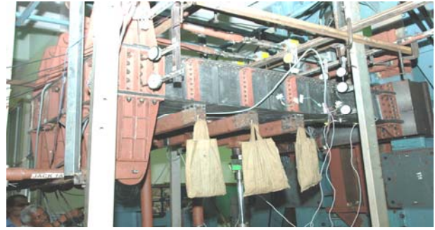
Fig. 36: Wing Test Box Undergoing Static Test
