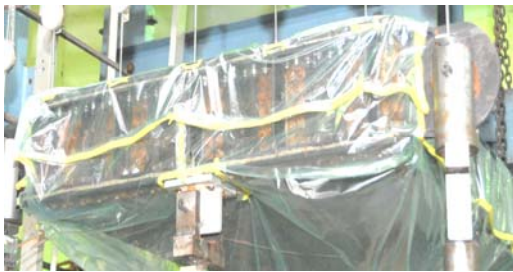
Fig. 12: Flexible Bagging Around the Box for the Steam
