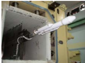
Fig. 3: Model in 1.2 m Trisonic Tunnel at NAL
