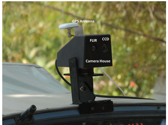
Fig-8 EVS prototype with stand mounted on test vehicle
