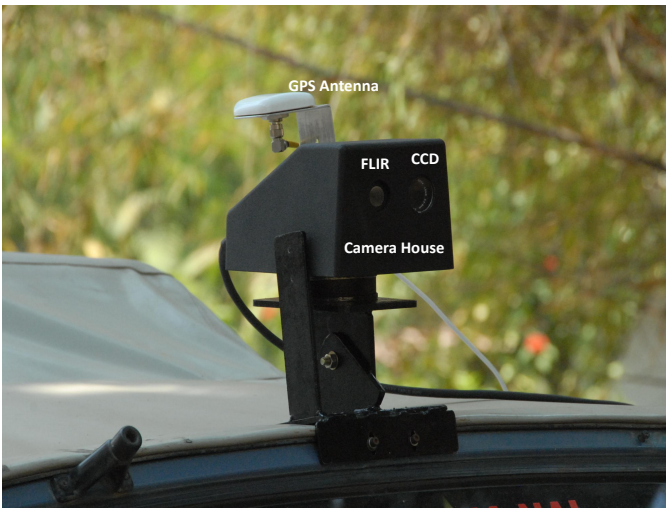
Fig. 8. EVS prototype unit with stand mounted on test vehicle
