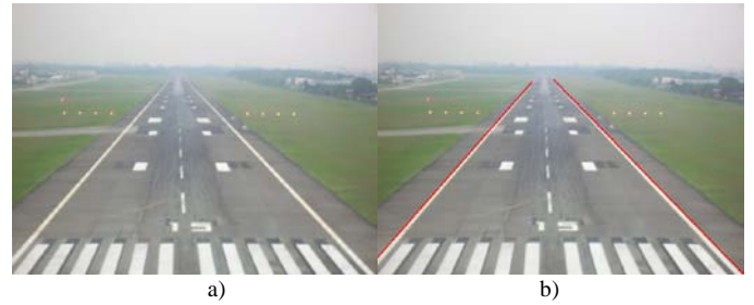
Fig.11: Test image 1a) Original image b) Extracted runway edges in red
