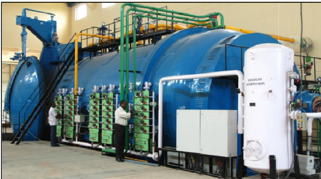
Figure 3. India's largest Aerospace Autoclave with working space of 4.4m dia x 9m length at CSIR-NAL, Bangalore
