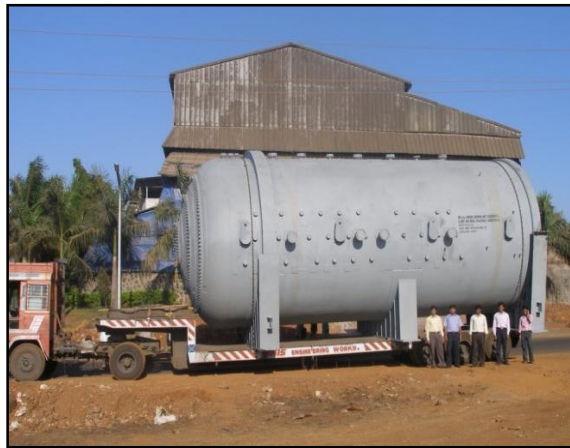
Figure 10. Transportation of the Autoclave shell
