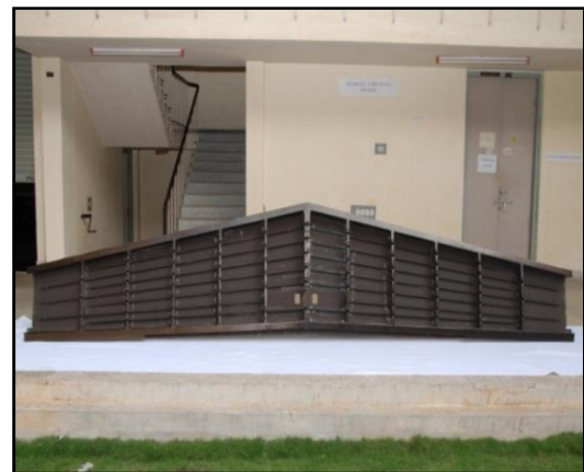
Figure 14. HT of SARAS aircraft, which was cured in an autoclave at NAL.
