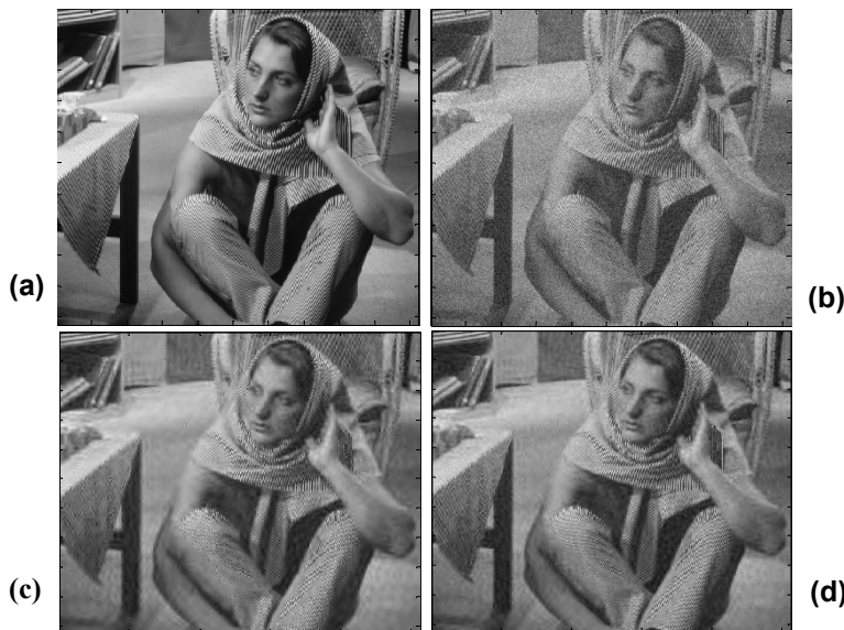
Fig.5 Denoising comparison for discontinuous signal (a) Clean (b) Noisy (10dB) (c) by DCHWT, O/P-SNR=13.1dB (d) ADCHWT, O/P-SNR = 13.7dB
