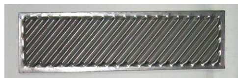
Figure-5a Single corrugated fin
