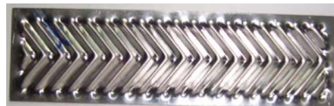
Figure-5b Double corrugated fin
