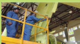
Calibration of trim tabs and FCS movement checks
