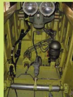
Hydraulic installation in NLG bay
