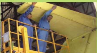
Calibration of trim tabs and FCS movement checks
