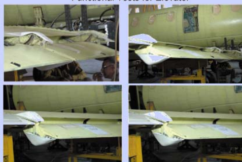
Functional Tests for Elevator
