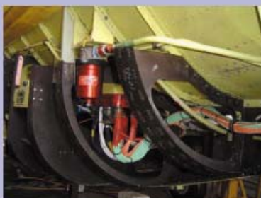
Fuel system in rear belly
