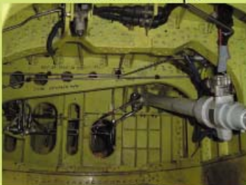
Hydraulic installation in MLG bay
