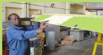
Calibration of trim tabs and FCS movement checks
