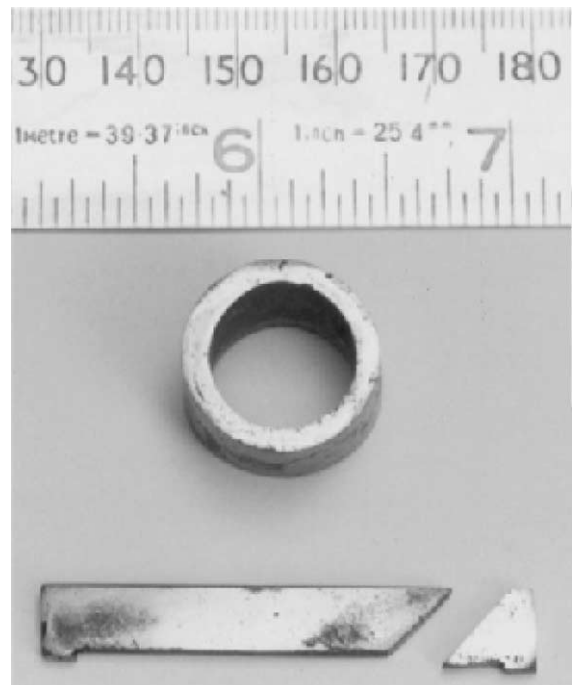
Fig. 7. Cylinder and seal fabricated using slip-casting technique.
