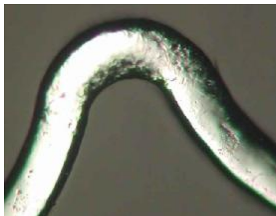
Fig. 2 Strain-lines of Tecnic Carbostent™, after expansion at 200 times magnification
