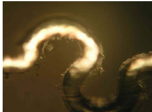
Figure 4. After expansion, the peeled off coating, N=100×
