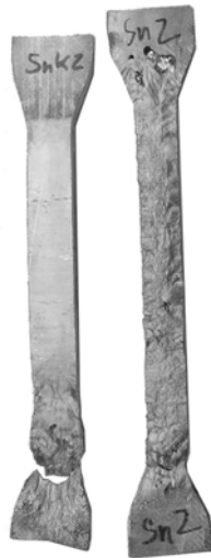
Figure 3. Composite wire reinforced tin matrix specimen (left) and pure tin specimen (right)
