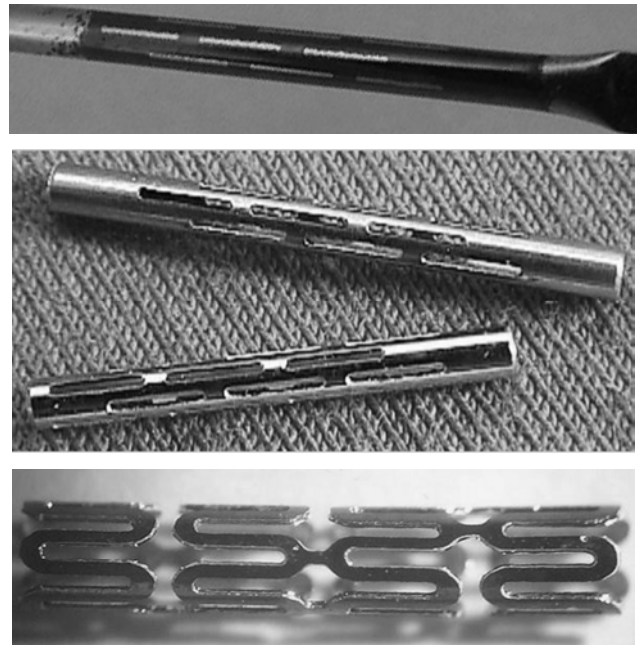
Fig.7: Processing sequences of BorGir ® Stent
