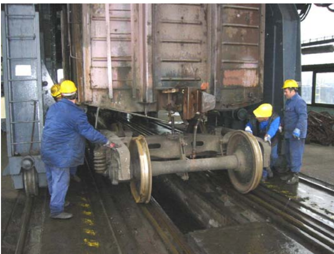
Figure 1 Treating interoperability discontinuity. Exchange of axles in Záhony
