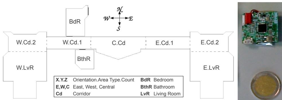
Fig. 1. Monitored areas of a single 45x20 m floor in a nursing home. The total monitored area is 307 m<sup>2</sup>. Dashed lines indicate virtual boundaries between areas, while solid lines indicate walls or doors. The photo shows a 2 euro coin and the mobile mote carried by the patients.
