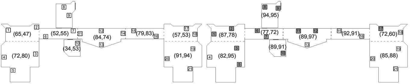
Fig. 2. Area accuracy for first (left) and second (right) deployments. Nodes moved between deployments are shaded in the second deployment. Values in parenthesis report the accuracy metric as (Max-RSSI, REWL).
