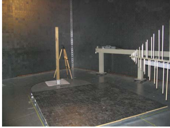
Figure 4 – Measurement set up of the anechoic chamber of the Joint Lab DIBE - EMC S.r.l., Genova, Italy.
