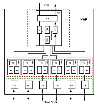
**Figure 2.1:** NWP block-diagram, on the green-dotted box are shown the PHY commodity components that manage the physical level of the links such as electrical signals; on the red-dotted box are shown the 6 link managers, together called TNW, that take care of the PHYs configuration and reliable data transfer. On the blue-dotted box is shown the interface to the CPU, called Input/Output Controller (IOC), it manages the PCIe link to the CPU and the DMA engine.
