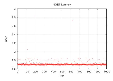
Figure 5.11: NGET latencies over 1000 measurements with delay=0 and payload=128B.
