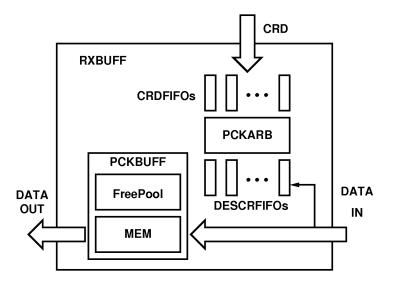
**Figure 2.11:** Detailed view of RXBUFF, credits provided by CPU are stored into the related CRDFIFO based on the virtual-channel they has been issued for, the incoming data are stored into MEM while the header (descriptor) is stored into the related DESCR-FIFO depending on the virtual-channel they belong, if the Packet Arbiter (PCKARB) find a match between one descriptor and one credit, the interface with the CPU is triggered to move data into main memory.
