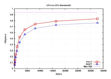
**Figure 5.16:** *CPU-to-CPU bandwidth measurements of PPUT and NGET methods, the purple line at 0.941 GBytes/s indicates the max usable bandwidth of the TNW link.*
