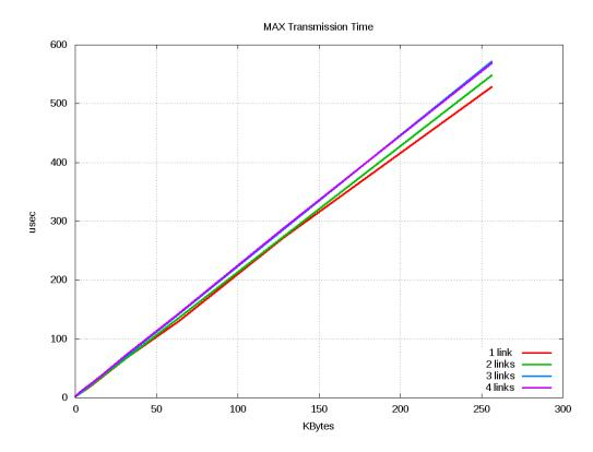
**Figure 5.25:** *Max Transmission time in micro-seconds* ( $\mu$ *sec*) *for one, two, three and four links active at the same time.*
