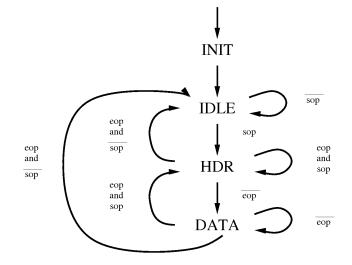
**Figure 3.8:** Diagram of the finite state machine RX\_FSM of the PIC module, it is controlled by the SOP and EOP signals exported by the PCIe Macro and allows to manage transactions with arbitrary payload size.
