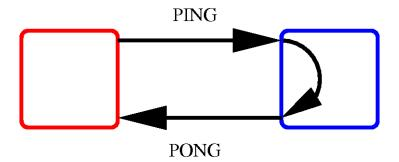
**Figure 4.6:** *Ping-pong Example, the red node sends a message (PING) to the blue one that, immediately send-it-back (PONG).*
