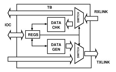
**Figure 2.12:** Block-diagram of the TB module. It's interposed between the CPU interface and the TNW's injection/reception buffers, when not enabled, the switches act like a pass through between IOC and TNW, so TB is completely transparent to the other modules, otherwise TB separates TNW from the CPU interface and manages autonomously the data-stream. All the TB's functionalities are fully controlled by register interface.
