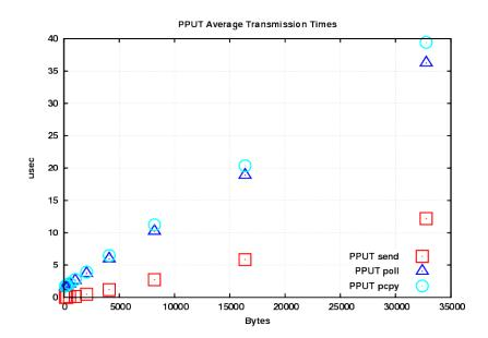
**Figure 5.19:** *CPU-to-CPU transmission times measurement of PPUT method, the red spots are the time to send data from CPU registers to PCIe, the blue ones include the time to send data over TNWs and DMA time to deliver to system memory, the light-blue include also the time to copy data from DMA buffer to USR buffer.*
