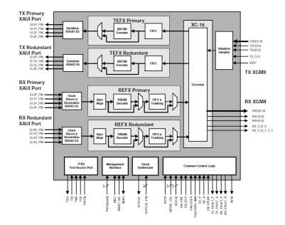
**Figure 2.3:** Block-diagram of the commodity PHY PMC-Sierra PM8358. On the leftside are visible the Primary/Redundant serial ports (XAUI) used for the node-to-node communications; on the right-side are visible the parallel ports (XGMII) managed by the TNW module.
