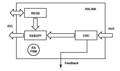
**Figure 2.10:** *Diagram of the RXLINK module. The lower section includes pipeline where data are checked using the CRC method and the reception buffer (RXBUFF) to store data before sending them to the CPU. The upper section is the register access.*
