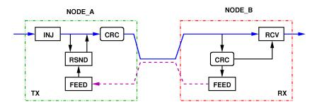
**Figure 2.2:** Node-to-node reliable communication diagram, it is based on a ACK/NAK protocol. Each packet is protected by a CRC and a copy of data is stored into the Re-send Buffer (RSND), if the CRCs on TX and RX match the packet is accepted issuing an ACK or otherwise it is discarded issuing a NAK. The ACK feedback removes the packet from RSND while a NAK implies the resend of the packet.
