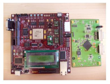
**Figure 5.1:** Hardware components for the BER test of the PM8354 PHY, on the left-side is shown the FPGA development kit while on the right-side is shown the PHY test-bed.
