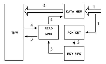
**Figure 3.9:** *Re-order Buffer scheme, data are stored into DATA\_MEM until completion* (1), *PCK\_CNT counts how many items of a packet are arrived* (1), *when done, the packet address is pushed into RDY\_FIFO* (2); *READ\_MNG interacts with TNW to send packets over the link* (3,4).
