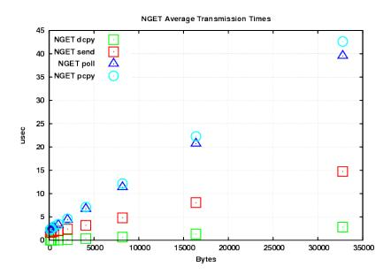
**Figure 5.21:** *CPU-to-CPU bandwidth measurement of NGET method, the green line is the time to copy data from USR buffer to DMA buffer, the red lines includes time to send data from CPU registers to PCIe, the blue one includes the time to send data over TNWs and DMA time to deliver them to system memory, the light-blue includes also the time to copy data from DMA buffer to USR buffer.*
