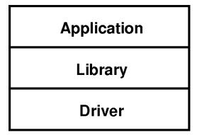
**Figure 4.1:** NWP software stack. The lowest layer is the Device Driver (DRV) who configures the network processors and allocates in main memory the required buffers. Over the Device Driver (DRV) is implemented the Low Level Library (LIB) who exports to the application all the basic routines to configure/monitor the network processor as well as the functions to send/receive data over links.
