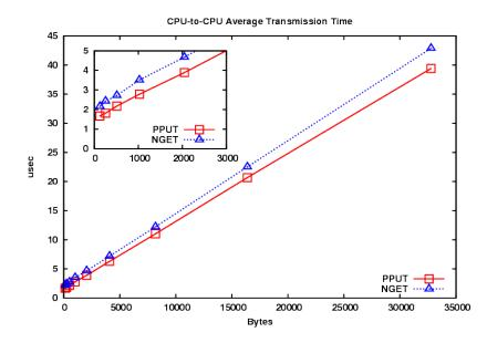
Figure 5.15: CPU-to-CPU transmission time measurement of PPUT and NGET methods.
