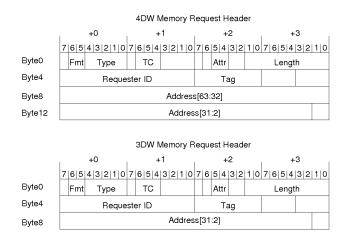
**Figure 3.4:** *PCI Express (PCIe) memory request headers, top-side shows the 4DW header used to operate on a 64-bit address-space, bottom-side shows the 3DW header used to operate on a 32-bit address-space*
