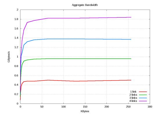
**Figure 5.26:** Aggregate Bandwidth for one, two, three and four links active at the same time.
