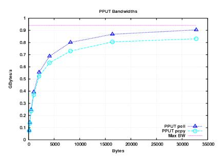
**Figure 5.20:** *CPU-to-CPU bandwidth measurement of PPUT method, the blue line shows the bandwidth achievable without considering the time to copy data from DMA buffer to USR buffer, that time is considered in the light-blue one. The purple line at 0.941 GBytes/s indicates the max usable bandwidth of the TNW link.*
