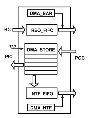
Figure 3.11: Diagram of the DMA engine.
