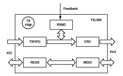
**Figure 2.6:** Diagram of the TXLINK module. The upper section is the data transmission pipeline, it includes the injection buffer (TXFIFO) and the modules to implement the custom packet-based ACK/NAK protocol, RSND stores packet-copies in case they must to be resent due to corruption among the link, CRC module computes the protection-code to validate or not the packet at the receiver-side. The lower section is the register access including the MDIO interface to the PHY.
