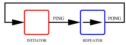
**Figure 5.23:** *Ping-Pong: INITIATOR sends a message to the REPEATER that sends it back.*
