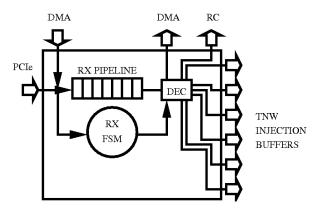
**Figure 3.7:** Conceptual layout of the PIC module, incoming packets are analyzed by the RX\_FSM and DEC to route the transaction to the right interface.
