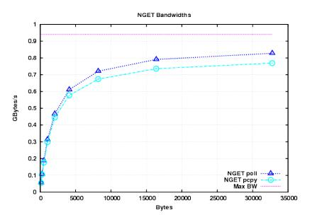
**Figure 5.22:** *CPU-to-CPU bandwidth measurement of NGET method, the blue line shows the bandwidth achievable without considering the time to copy data from DMA buffer to USR buffer, that time is considered in the light-blue one. The purple line at 0.941 GBytes/s indicates the max usable bandwidth of the TNW link.*
