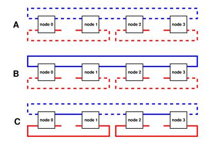
**Figure 2.4:** *Re-partitioning example of a four-nodes machine. Depending on configuration of PHY ports, primary (blue lines) or redundant (red lines), the machine can be configured as one four-nodes machine (layer "B") either as two separated two-nodes machines (layer "C") without re-cabling the connections.*
