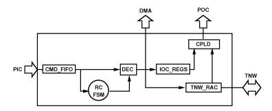
Figure 3.10: Diagram of the Register Access Controller.
