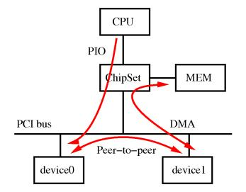
**Figure 3.3:** PCI transaction modes, in PIO mode both CPU and target device are involved until the end of the transaction, data are transferred from the internal registers of the CPU to the address-space of the target device. In DMA the device directly access the memory without CPU intervention, just interacting with the memory controller, letting the CPU freely computing. In Peer-to-peer mode a master device can autonomously access a target device.
