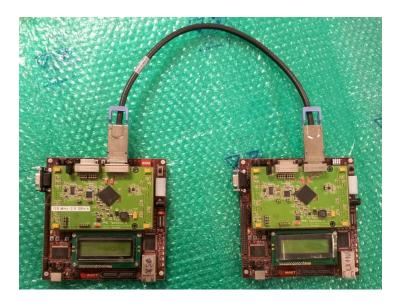
**Figure 5.2:** The dual end-point setup for the BER test. Here two FPGA development kits are equipped with the PHY test-beds and connected by a 50cm cable. Each FPGA has been programmed with the test bench firmware for the full-duplex communications. This setup has been used for an extensive campaign with many runs up to 21 days of bidirectional transmissions without any error detected.
