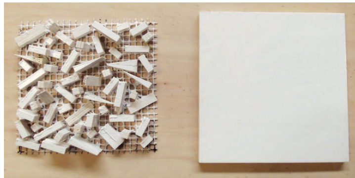
Figure 3.15: Materials tested inside the reverberation chamber: a patch of varnished scattering elements (on the left) and a flat varnished tile (on the right).
