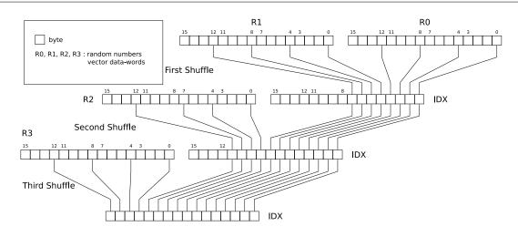
Figure 4.12: The shuffling of  $V_r \times 32$ -bit random numbers, to compose the vector data-word IDX that is used to perform comparison with the energy differences vectors.
