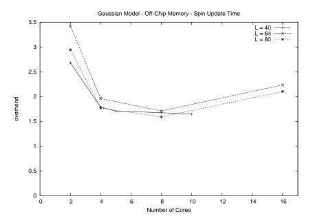
Figure 5.9: System Spin update time  $\tau(V)$  as a function of the number of cores C for several linear lattice sizes L.
