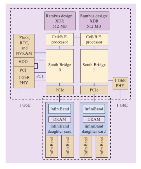
Figure 1.7: The organization of a QS21 Blade Server. Note that the two processors are directly connected and that, although some resources are shared (as the PCI interface), each processor has its own XDR memory, Gbit PHY and PCI interfaces. Figure is from [39].
