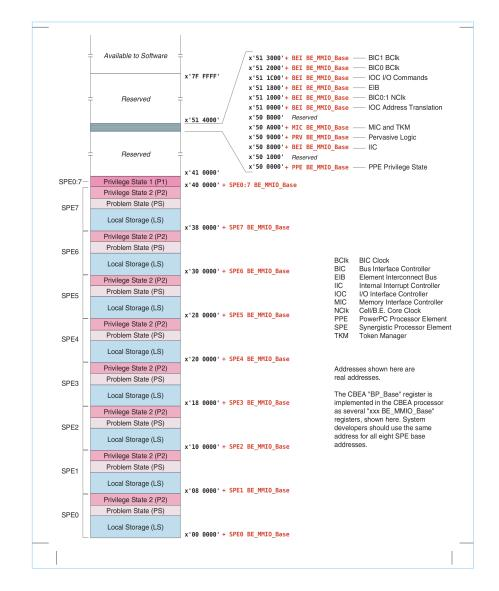
Figure 1.6: An overview of the mapping of SPEs resources into effective address space. Figure is from [36].
