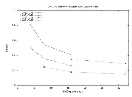
Figure 5.3: The system Spin update time  $\tau(V)$  as a function of SIMD-granularity V for several linear lattice sizes L and number of cores C.
