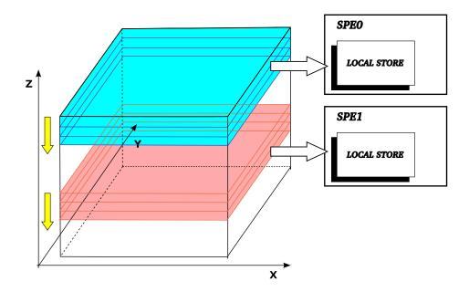
Figure 3.5: Each cores has to update a sublattice of L/C XY-planes that is too large to be stored in local memory. Instead, a set of half-planes is loaded from main to local memory to update a single half-plane.
