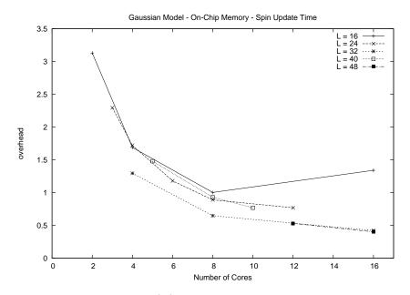
Figure 5.8: System Spin update time  $\tau(V)$  as a function of the number of cores C for several linear lattice sizes L.
