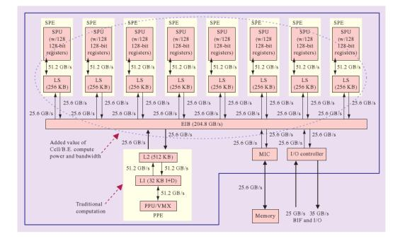
Figure 1.4: Block diagram of the CBE processor. Figure is from [32].
