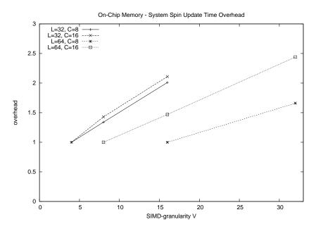
Figure 5.4: The overhead of the system Spin update time  $\tau(V)$  in to respect of the ideal one (assuming perfect scaling) as a function of SIMD-granularity V for several linear lattice sizes L and number of cores C.
