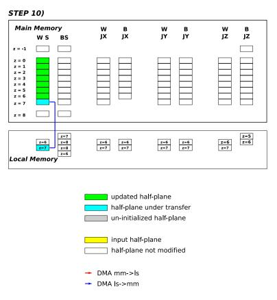
Figure 4.18: The final step of the update of the half-planes of a core. All the half planes have been updated and the last one is stored back to main memory.
