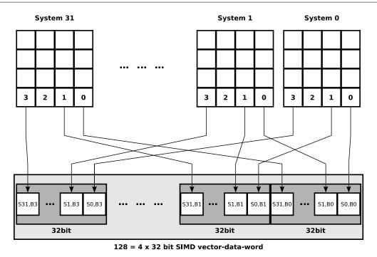
Figure 3.1: An example of the mapping of w = 32 different systems into one W = 128-bit SIMD vector data-word. Each vector represent V = 4 spins of each system.
