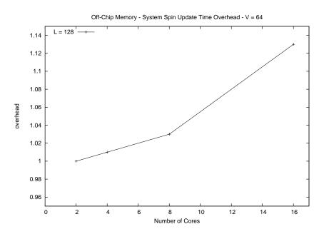
Figure 5.7: The system spin update time overhead as a function of the number of cores C with fixed SIMD-granularity V = 64 and lattice linear size L = 128.
