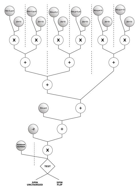
Figure 4.13: The DAG of the spin update procedure. Note that the dotted lines indicate operations that can in principle be executed in parallel, so that instruction level parallelism can be exploited.
