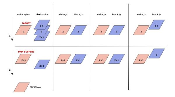
Figure 3.6: The buffers that have to be used to update a half plane while storing back a previously update half-plane and loading from main memory the data required to update the next half plane
