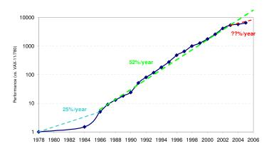
Figure 1.2: The improvements of computing power of processors in the last 30 years (This figure is Figure 1.1 in [17].
