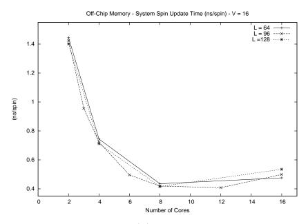
Figure 5.5: The system spin update time  $\tau(V)$  as a function of the number of cores C with fixed SIMD-granularity V = 16 and for several lattices sizes L.
