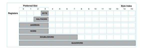
Figure 1.3: The SIMD-granularities supported by CBE. Note that each type of instructions supports only specific types of variables. For example, single-precision floating-point instructions supports only the "word" (four 32-bit scalar variables) granularity. (Figure is from [31])
