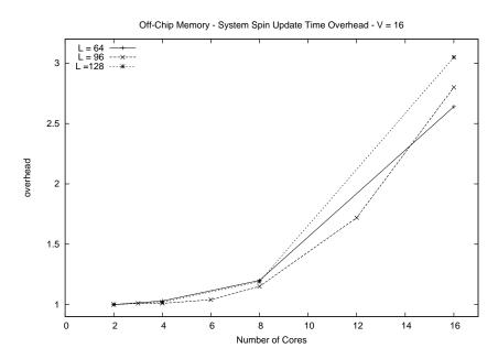
Figure 5.6: The system spin update time overhead as a function of the number of cores C with fixed SIMD-granularity V = 16 and for several lattices sizes L.
