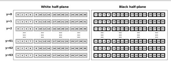
Figure 4.1: Distribution of the spins of a plane among vector data-words. The numbers inside the square indicate the X coordinates of the w spins embedded in that scalar element.
