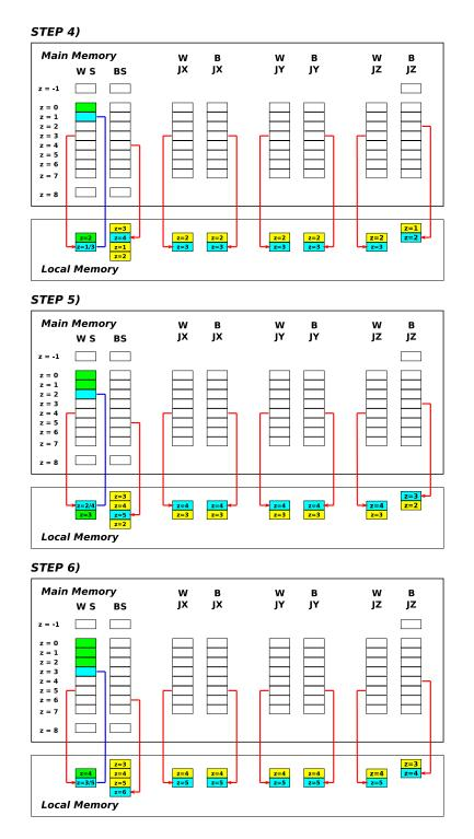
Figure 4.16: Steps 4,5 and 6 of the update of the half-planes of a core. This is the most common case: while a half-plane is updated, 9 half-planes are concurrently exchanged with main memory.
