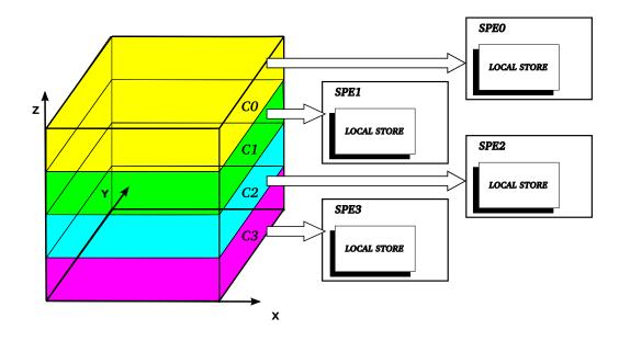
Figure 3.4: Each core loads into its local memory a sub-lattice of L/C XY-planes and some additional border data. The sums of all the local memories allows to store the representation of the whole lattice.
