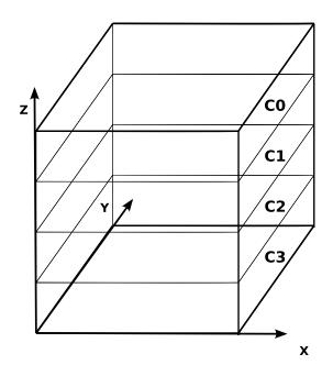
Figure 3.2: The cubic lattice is subdivided in sub-lattices of L/C XY planes, and each sub-lattice is assigned to a different core. Note that in this figure each element of the lattice represents both spins and couplings.
