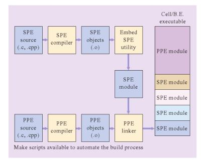
Figure 1.8: The compile chain of CBE. Note that the executable of PPE and SPEs are compiled independently, and that only in the linker phase are united into a single executable file. Figure is from [39].
