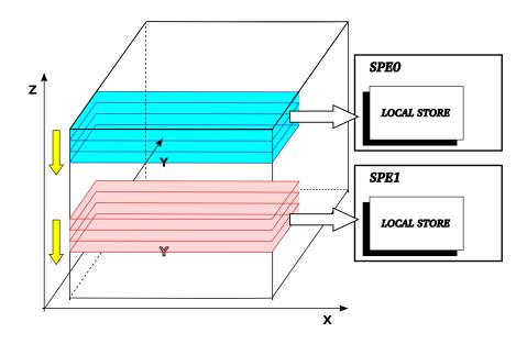
Figure 3.7: A sub-lattice of L/C XY-planes is assigned to each cores. Half-planes are subdivided in slices that are sequentially updated by the core in charge for that half-plane.
