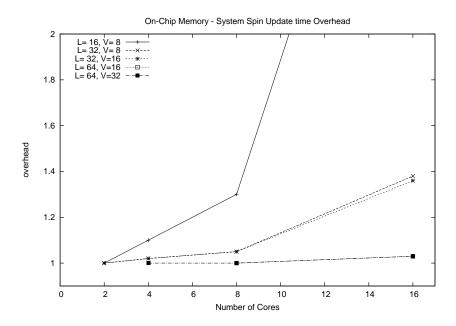
Figure 5.2: The overhead of the system Spin update time  $\tau(V)$  in to respect to the ideal one (assuming perfect scaling) in function of the number of cores C for several linear lattice sizes L and SIMD-granularities V.
