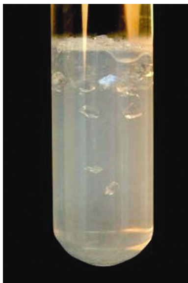
Figure 1. Growth of sodium oxalate monohydrate crystals in silica hydro-gel.
