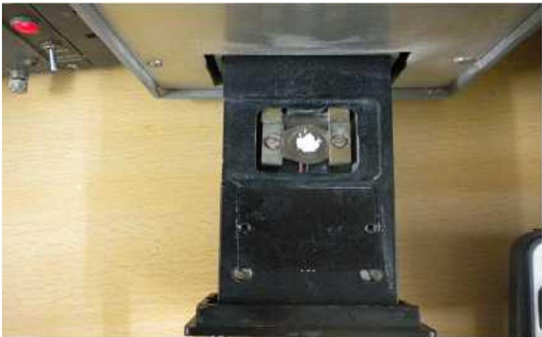
Fig. 3.12: Kanthal Strip and TL detection head
