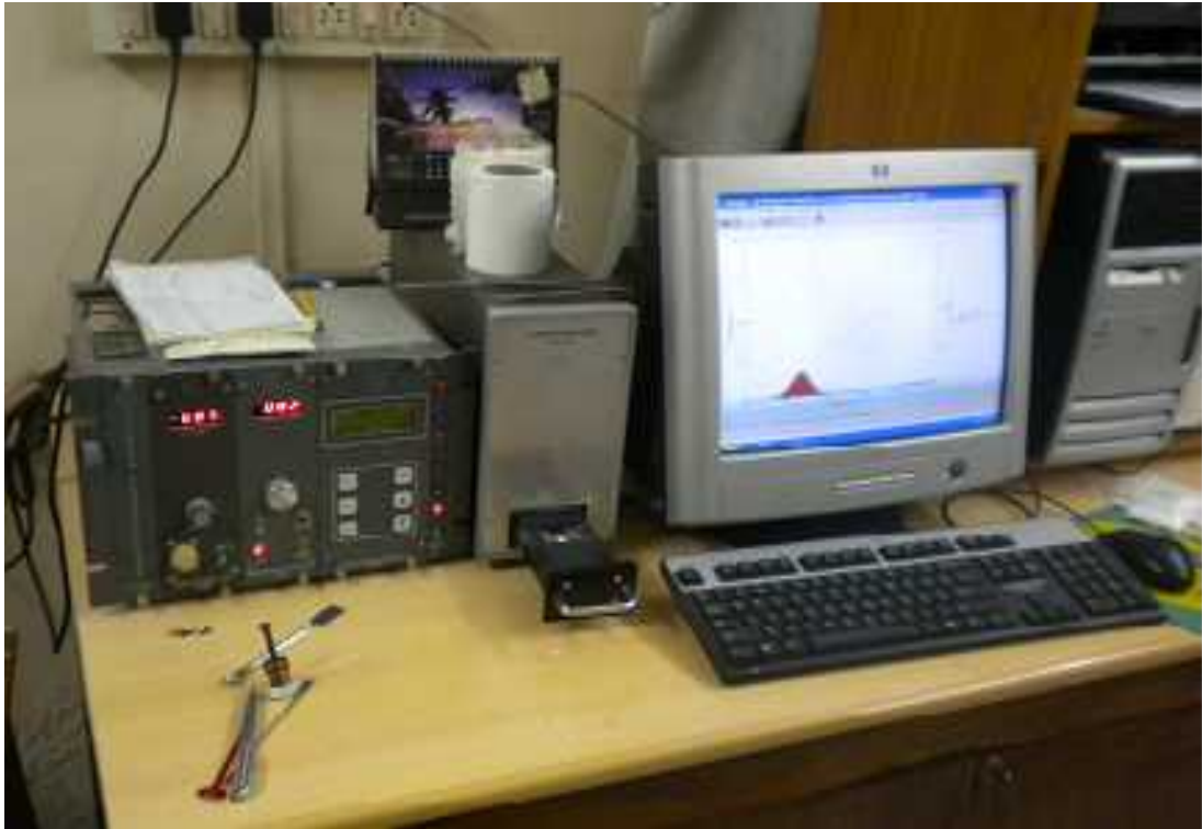
Fig. 3.11: TL Reader set-up
