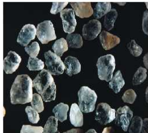
Fig.1.3: A microscopic view of sand grains in sediment shows the effects of transportation by running water. The grains are rounded and sorted to approximately the same size.
