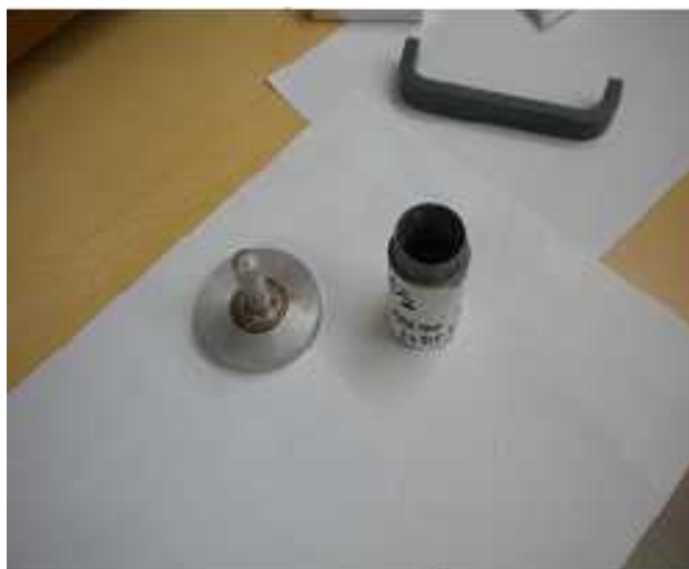
Fig. 3.10: Irradiation process by Sr^{90} beta source
