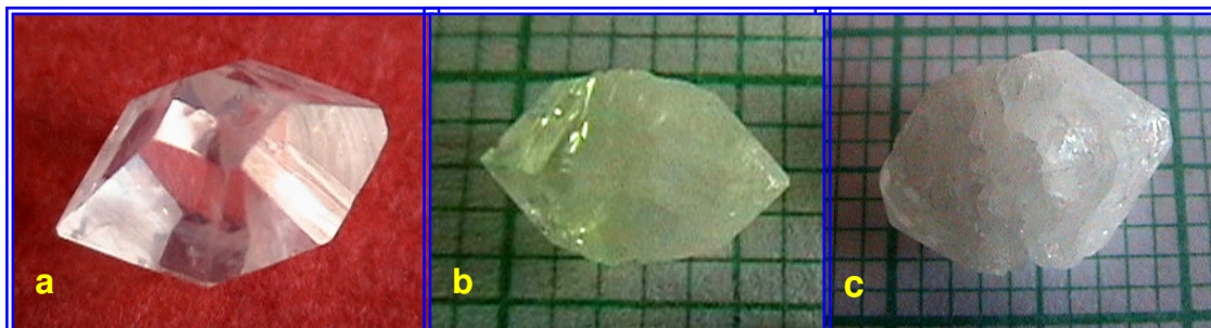
Figure : 5.11 Different Diaphaneity of Prismatic Type Struvite Crystals (a) Transparent, (b) Translucent and (c) Opaque
