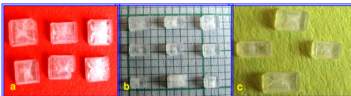
Figure : 5.6 Rectangular Platelet type Struvite Crystals with Growth Parameters SMS of SG 1.06, 0.75 M ADP, 0.75 M SS for (a) 7.2 pH; (b), (c) 7.5 pH values of gel
