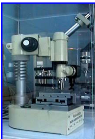
Figure : 7.7 Vaiseshika Vickers Micro-hardness Tester Type 7005
