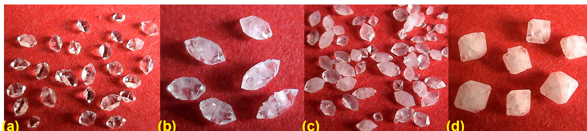
Figure : 8.7 Prismatic Type Struvite-Na Crystals Grown with the Conditions as 1.05 SG of SMS, 0.5 M SDO, 0.5 M SS and pH Value of Gel as (a) 6.0 pH, (b) 6.5 pH, (c) 7.0 pH and (d) 7.5 pH
