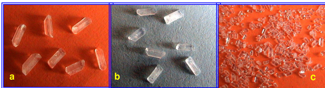
Figure : 5.7 Coffin Shaped Struvite Crystals for the Growth Parameters (a) and (b) SMS of SG 1.06, 1.0 M ADP, 1.0 M SS for 7.0 pH value of gel; (c) SMS of SG 1.06, 0.75 M ADP, 0.75 M SS for 8.0 pH value of gel
