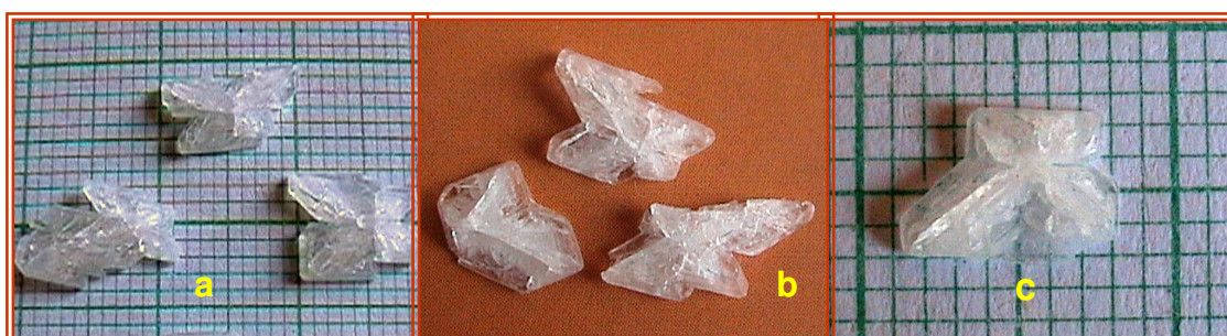
Figure : 5.9 Branched Dendritic type Struvite Crystals with Growth Parameters
