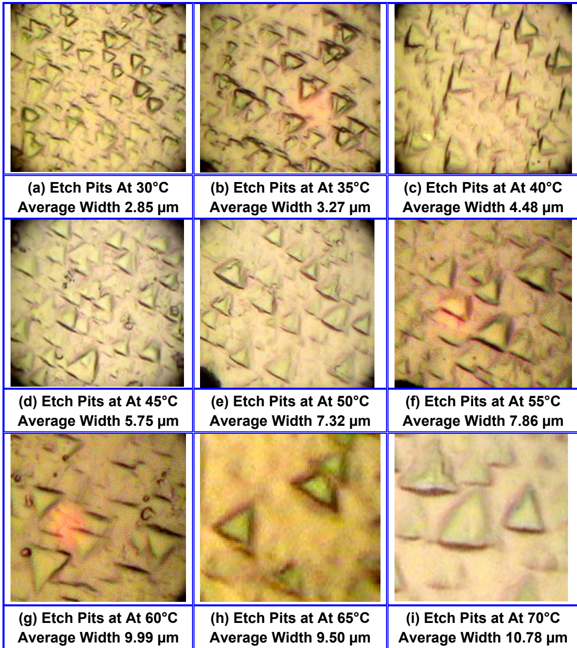
Figure : 7.13 Triangular Etch Pits Observed on (111) Face of the Struvite Crystals
