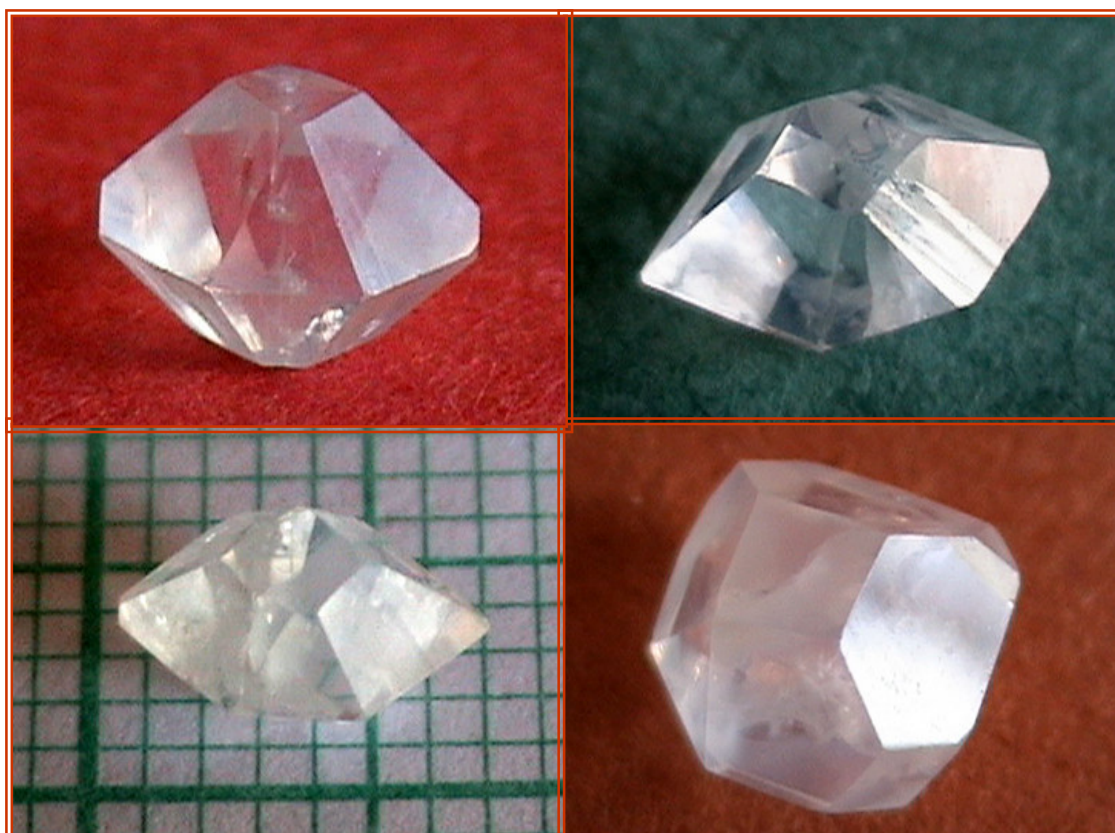
Figure : 5.2 Prismatic Type Struvite Crystals Grown for the Growth Parameters as SMS of SG 1.04, 1.0 M ADP, 1.0 M SS with 7.0 pH Value of the Gel
