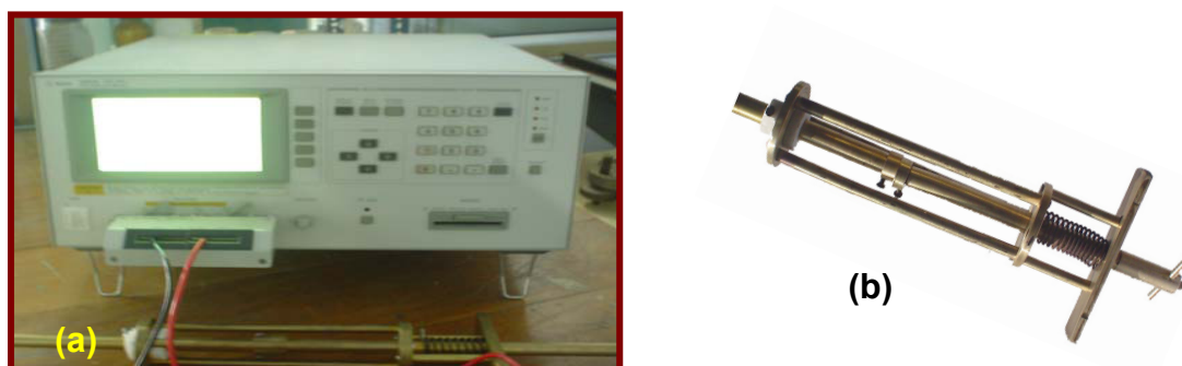
Figure : 4.11 (a) Agilent 4284 A precession LCR meter (b) Sample Holder
