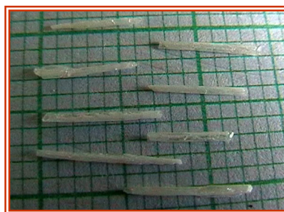
Figure : 5.10 Needle Type Struvite Crystals with Growth Parameters SMS of SG 1.06, 0.5 M ADP, 1.0 M SS for 10.0 pH value of Gel
