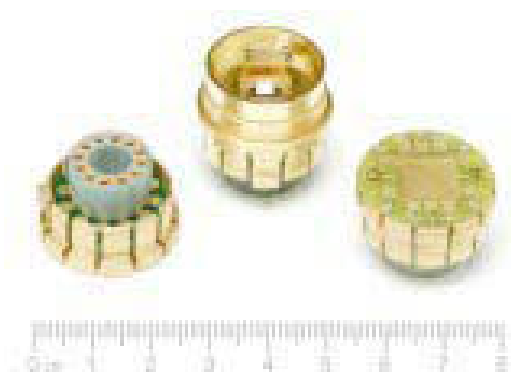
Figure 3.13 Specialized pucks, 2.4 cm in diameter, are used for different measurement applications.
