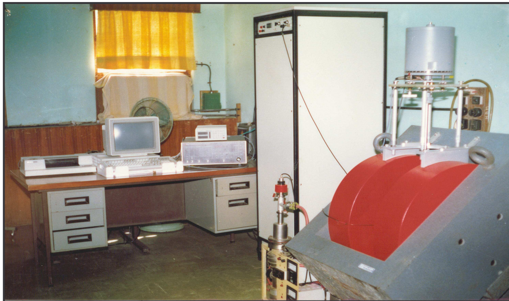
Fig.14 Fully computer – controlled vibrating sample magnetometer (EG&G PARC Model 4500)
