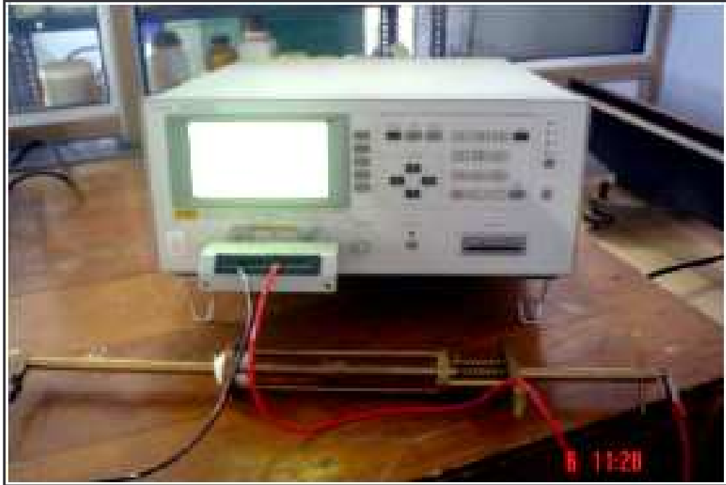
Fig.33 A photograph of Impedance analyzer (4284 A) and sample holder used in present investigation
