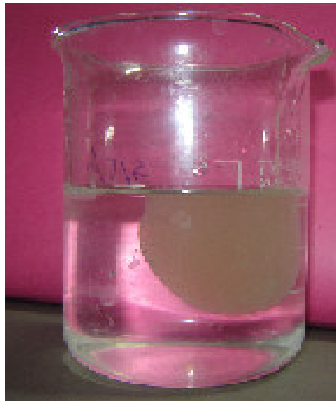
Figure 5.3: Gel formation of alginate based in situ gel in simulated gastric fluid (batch F5)
