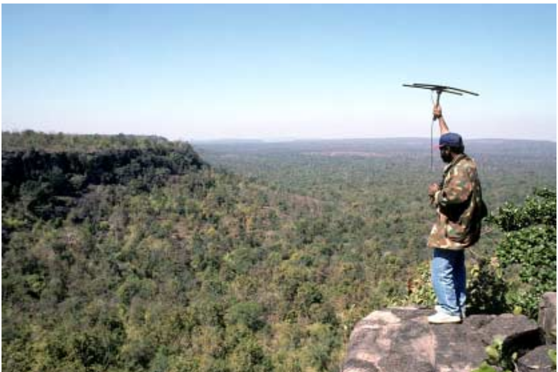
Plate 4b. Using mobile receivers and hand-held antennas, radio-tagged bears were tracked in Panna NP for many years. Radio signals were obtained from vantage points like this ledge, and were approached closer or their locations were estimated by method of triangulation. (Photo courtesy: Cliff Rice).
