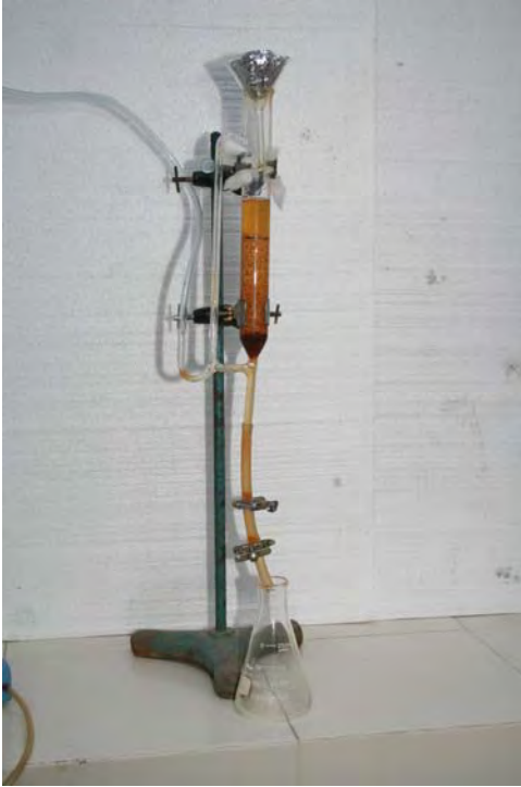
Photograph 12. Laboratory scale column reactor for copper bioremoval (A) citrate broth with Enterobacter sp. (B) polystyrene beads after biofilm formation.
