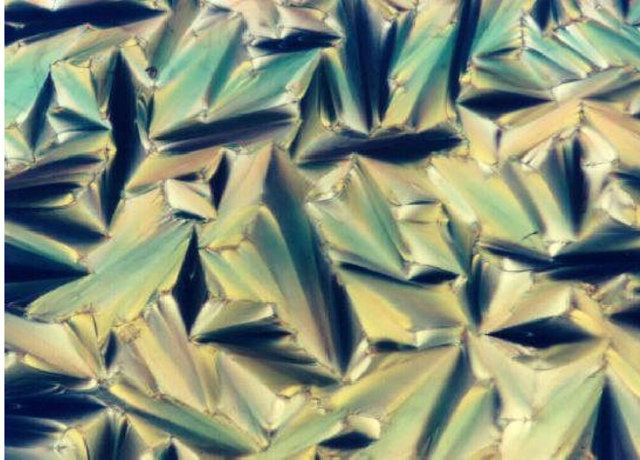
Fig. 9(a) Texture of the Smectic liquid crystal phase
