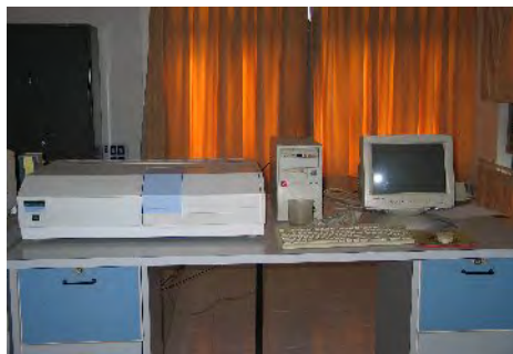
Figure :6.7 A photograph of typical set up of UV-Vis spectrophotometer.
