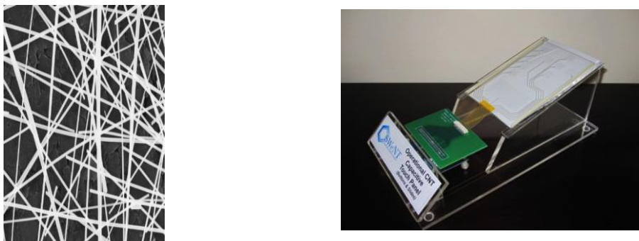
Figure 2: (left) Silver nanowire transparent electrodes. (right) An example of a carbon nanotube touch screen.
