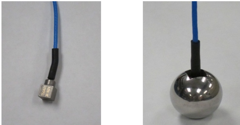
Figure 2.5: In-situ accelerometer sensor. (left) Photograph of the accelerometer. (right) Photograph of a steel sensor particle (accelerometer embedded in a drilled steel sphere).
